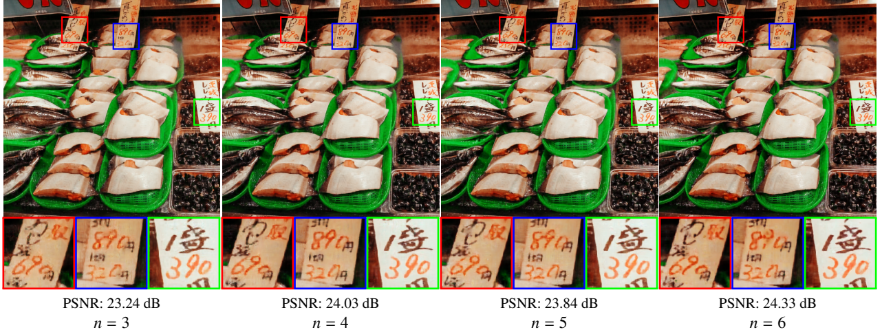
Figure 2: Qualitative comparison of various n -values with N = 64 for the FISH MARKET image.
