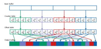
Figure 1: Parallel radix sort using four threads.
