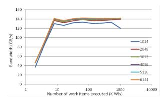
Figure 2: The effective bandwidth on AMD Radeon HD5780 (Theoretical peak bandwidth is 153.6GB/s).
