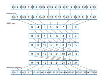
Figure 3: Parallel scan algorithm.
