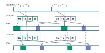
Figure 4: The reordering step. It illustrates two steps of a local sort and a write. A SIMD engine reads 256 keys and sorts locally and write them back to memory.
