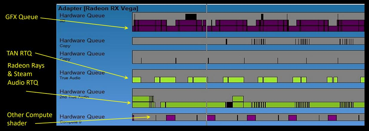
This Windows Performance Recorder capture trace (as seen in GPUView) shows four queues running independently on one GPU, in a Direct X<sup>®</sup> 12 scenario: TAN, Radeon Rays, 3D graphics, and a gaming compute shader process
